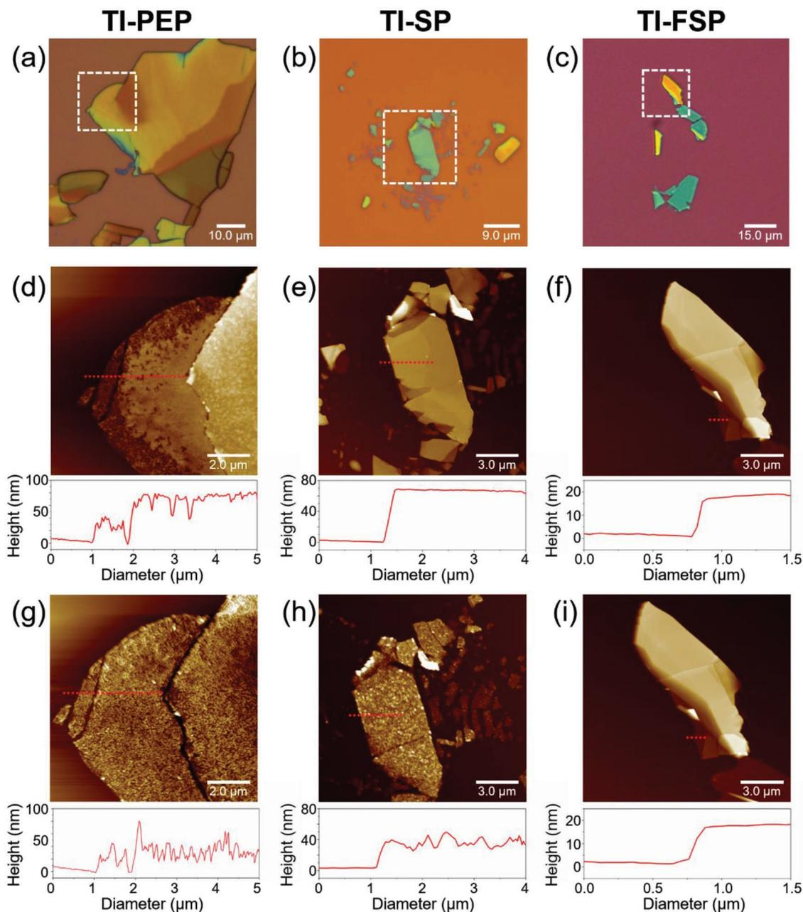
**Figure 6.** Optical images of a) **TI-PEP**, b) **TI-SP**, and c) **TI-FSP**. Time-dependent stability of exfoliated, tin-based perovskites multilayers prepared by the scotch-tape method from their bulk single crystals AFM images and corresponding height profiles of the exfoliated flakes of d) **TI-PEP**, e) **TI-SP**, and f) **TI-FSP**; and after exposure in ambient condition for g) 6 h, h) 24 h, and i) 24 h, respectively.
