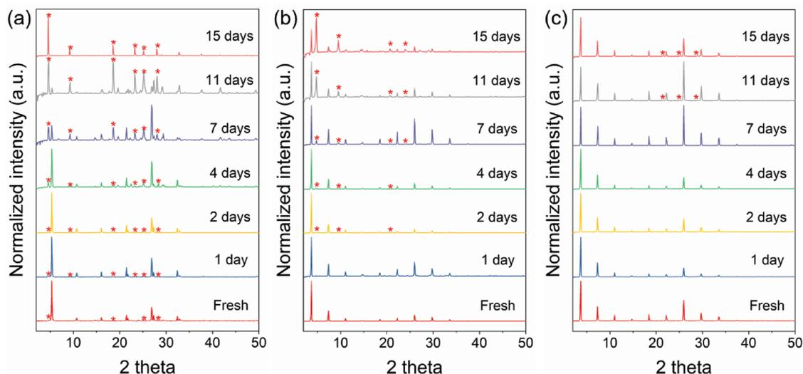
**Figure 5.** Air-stability of tin(II) iodide perovskites: comparison of PXRD patterns of a) **TI-PEP**, b) **TI-SP**, and c) **TI-FSP** for the fresh perovskites and after exposure to ambient condition at 60% RH for up to 15 d (\*: oxidized products).
