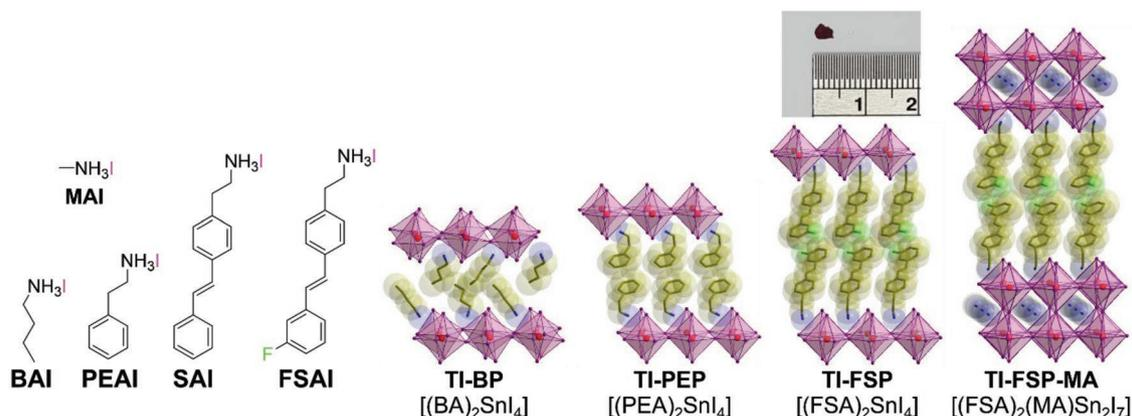
**Figure 1.** Chemical structures of the amine derivatives and their tin(II) iodide perovskites.
